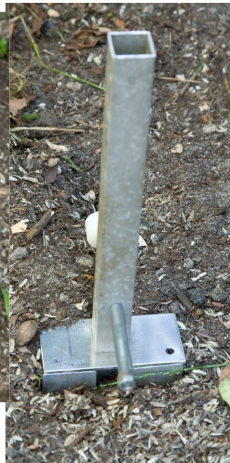
Monopod drilled down to bury resistance plates.
