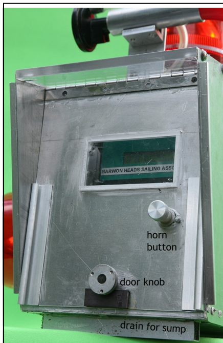
Figure 7: operator's access door has a magnetic catch (don't turn knob).
