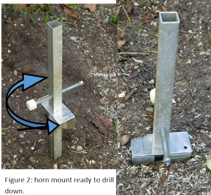
Monopod drilled down to bury resistance plates.
